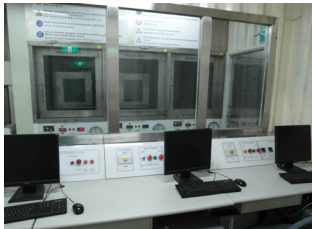
T.5 External Short Circuit
