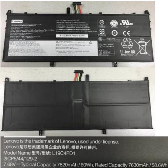
7.680 --- Typical Capacity 7820mAh / 60Wh, Rated Capacity 7630mAh / 58.6 额定容量: 7630mAh 充电限制电压(limited charging voltage): 8.8V For use with Lenovo personal computer
