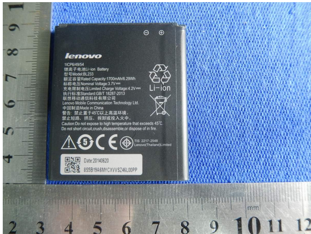
Battery (BL233 3,7V 1700mAh 6,29Wh)
