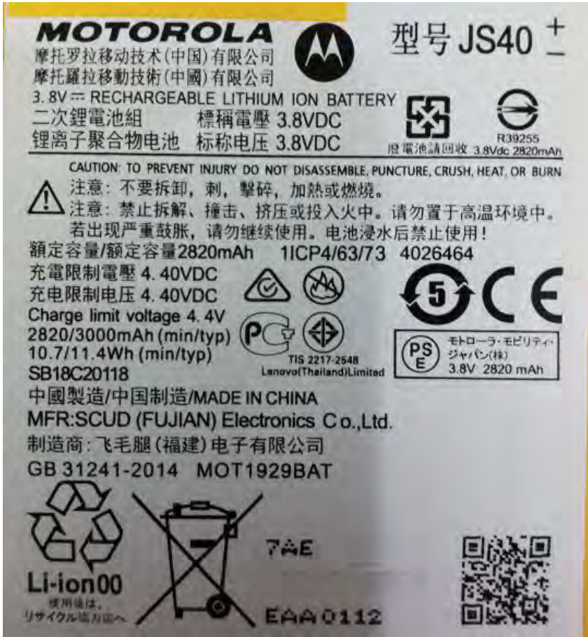
电池组铭牌 Battery Nameplate
